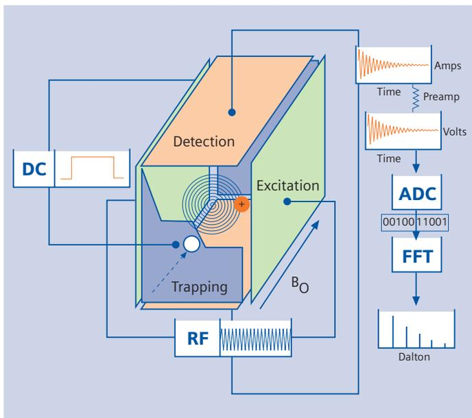
Figure 3: Measurement cell
