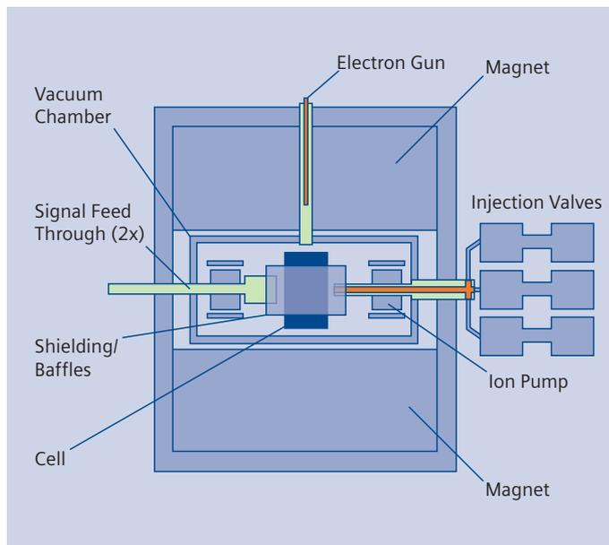
Figure 11: Schematic of the measuring chamber
